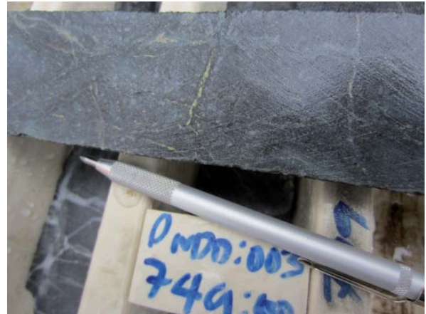
Figure 4: PNDD003; 749m. Fine chalcopyrite vein stockwork and disseminations, with biotite alteration forming vein selvages. The sample is characteristic of outer potassic alteration off the margin of a big porphyry Cu-Au-Mo system.
